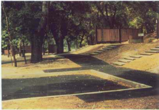
This southern California campground illustrates site hardening appropriate to an Urban facility. Curb cuts and a ramp to each unit should be provided for disabled campers.
